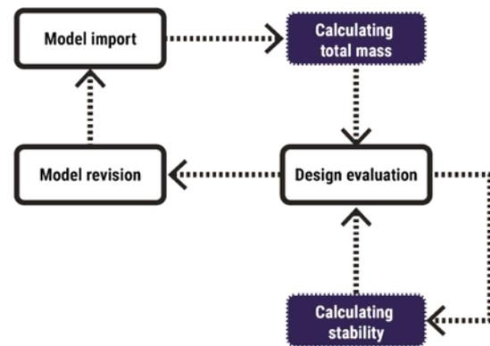
Fig. 2. Stability simulation process workflow; source: own elaboration
