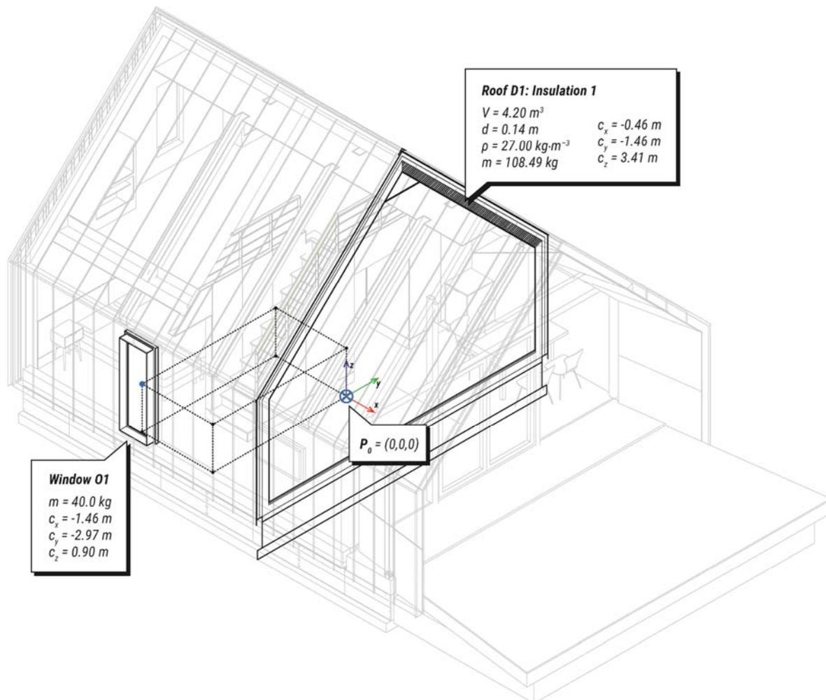
Fig. 3. Axonometric scheme of the geometry analysis;  $V$  = volume,  $d$  = layer thickness,  $\rho$  = material density,  $m$  = mass,  $c$  = center of mass,  $P_0$  = model origin; source: own elaboration
