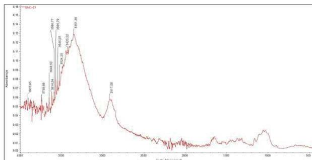
FIG. 1. IR spectra of BNC covered with gelatin.
