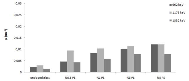
Fig. 4. The measured  $\mu$  for the soda-lime-silica glasses doped with the peanut shell powders at energies of 662, 1173 and 1332 keV.
