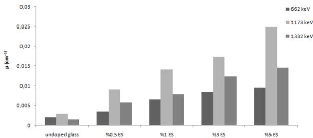
Fig. 3. The measured  $\mu$  for the soda-lime-silica glasses doped with the egg shell powders at energies of 662, 1173 and 1332 keV.
