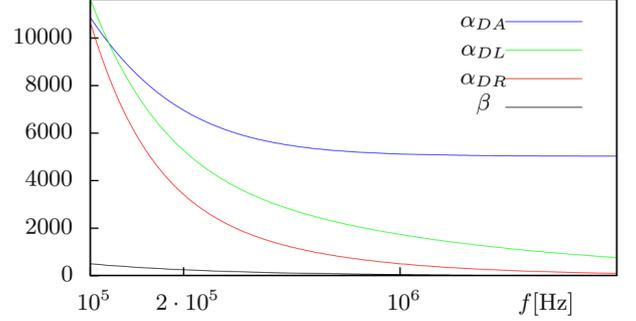
Fig. 2. Plots of the constants  $\alpha$  and  $\beta$  of Eq. (8) as a functions of the wave frequency at  $r = 4 \times 10^{-6}$  m radius of the cell. The symbols  $R$ ,  $L$ ,  $A$  distinguish the types of drift.
