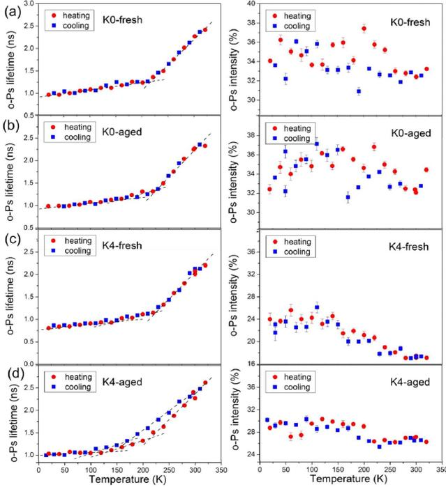
Fig. 2. *o*-Ps lifetime  $\tau_3$  (left) and intensity  $I_3$  (right) versus temperature for (a) K0-fresh, (b) K0-aged, (c) K4-fresh, and (d) K4-aged polymers. The samples are marked as shown in Fig. 1. The error bars for *o*-Ps lifetime data are within the size of the symbol. The dashed lines are drawn as a guide for the eye.
