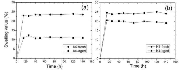
Fig. 3. Swelling value versus time curves for (a) K0-fresh and K0-aged and (b) K4-fresh and K4-aged polymers in EtOH at room temperature. The samples are marked as shown in Fig. 1. The error bars are within the size of the symbol.
