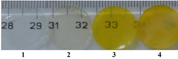
Fig. 1. Images of the investigated polymers used for the research: 1 — ureasil fresh (2 months after preparation): K0-fresh, 2 — ureasil aged (1 year after preparation): K0-aged, 3 —  $\text{As}_2\text{S}_3$ + ureasil fresh (2 months after preparation): K4-fresh, 4 —  $\text{As}_2\text{S}_3$ + ureasil aged (1 year after preparation): K4-aged.
