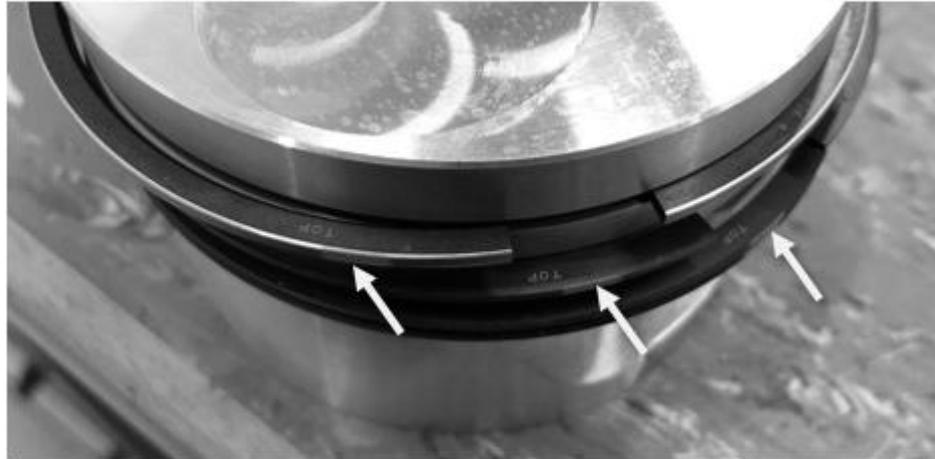
Fig. 1. Piston with incorrectly installed sealing rings
