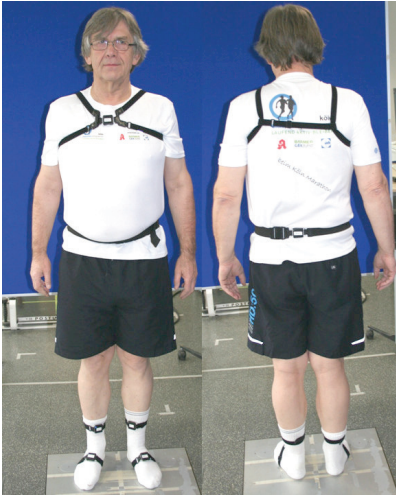
Figure 2. Movement sensor positions for balance ability measurement
