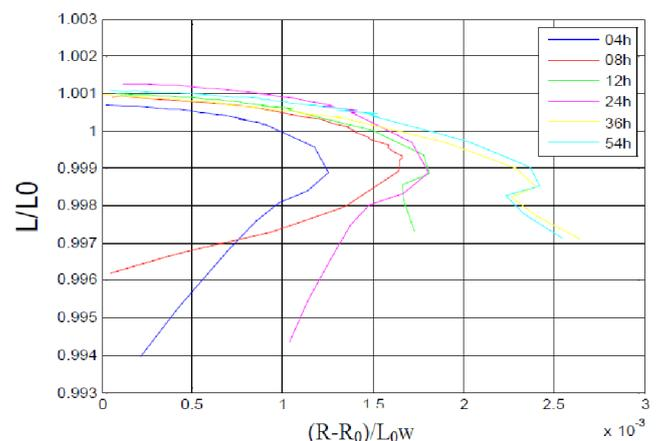
Fig. 1. The impedance diagrams of  $\text{Cu}_{70}\text{Co}_{30}$  for different milling times.
