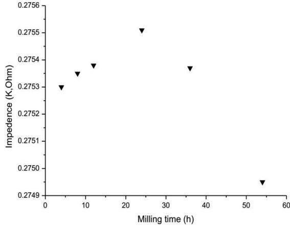
Fig. 2. Variation of the impedance as a function of milling time in  $\text{Cu}_{70}\text{Co}_{30}$ .
