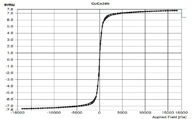
Fig. 4. The shape of the hysteresis curves recorded for the sample milled for 24 h.
