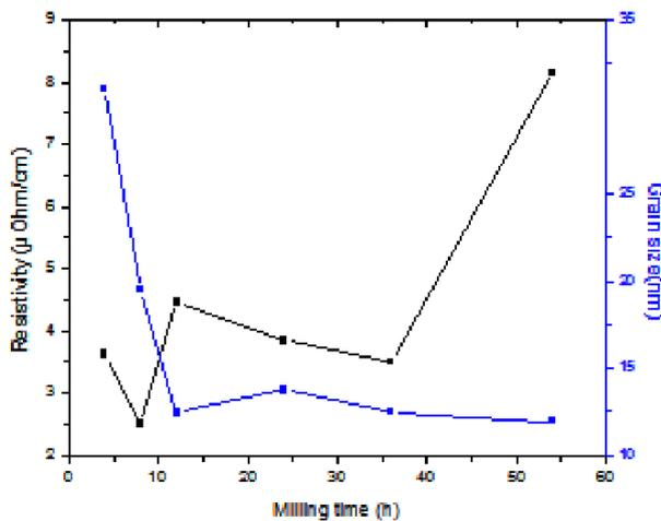
Fig. 3. Crystallite size and resistivity evolution as a function of milling time for  $\text{Cu}_{70}\text{Co}_{30}$ .
