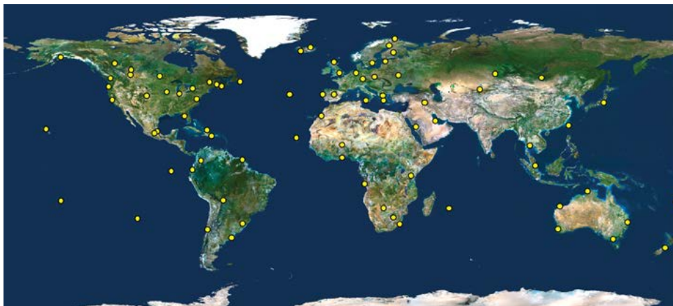
Fig. 1. Diagram of CenterPoint RTX control stations distribution (Leonardo et al., 2011)
