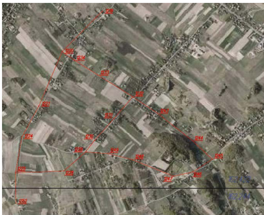
Fig. 5. The outline of detailed control network class III (test control network) on the object of „Jerzmanowice-Przebinia”
