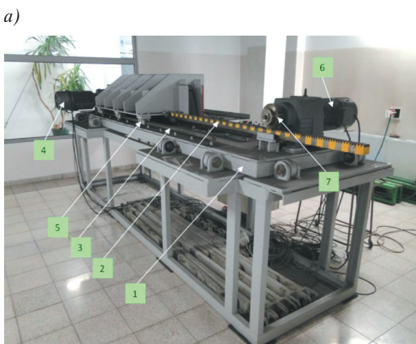
Fig. 4. Station for testing loading process: a) view of test bench from side of feed motor and rail; b) view from drum: 1 – station base, 2 – toothed rack, 3 – guide rails, 4 – drum drive motor, 5 – sliders, 6 – feed drive motor, 7 – gear cog, 8 – cutting drum, 9 – sliding frame
