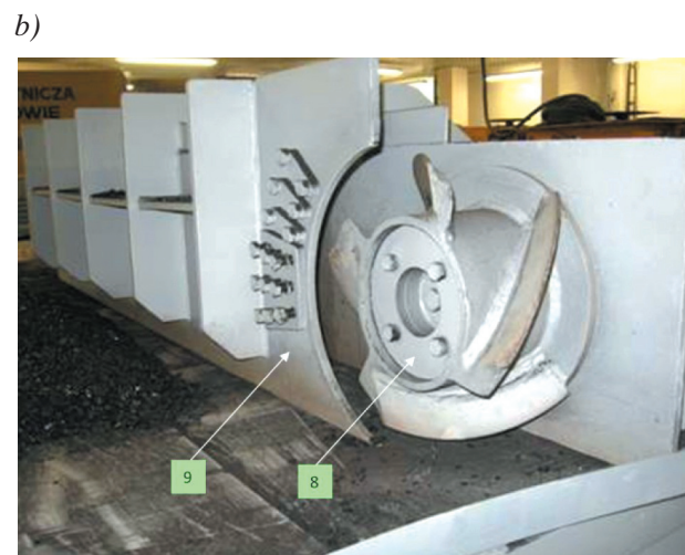
Fig. 4. Station for testing loading process: a) view of test bench from side of feed motor and rail; b) view from drum: 1 – station base, 2 – toothed rack, 3 – guide rails, 4 – drum drive motor, 5 – sliders, 6 – feed drive motor, 7 – gear cog, 8 – cutting drum, 9 – sliding frame
