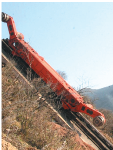
Fig. 3. Classic longwall shearer for strongly inclined seams at testing grounds of Beijing HOT Mining Tech [5]
