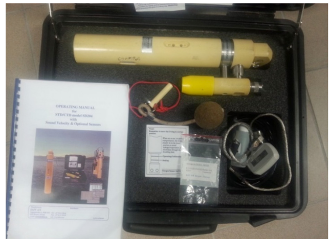
Fig. 2. CTD/STD probe (model SD204 by the SAIV AS company) used in the registrations
