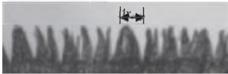
Figure 10. Graphical definition of  $\Delta x_{chip}$
