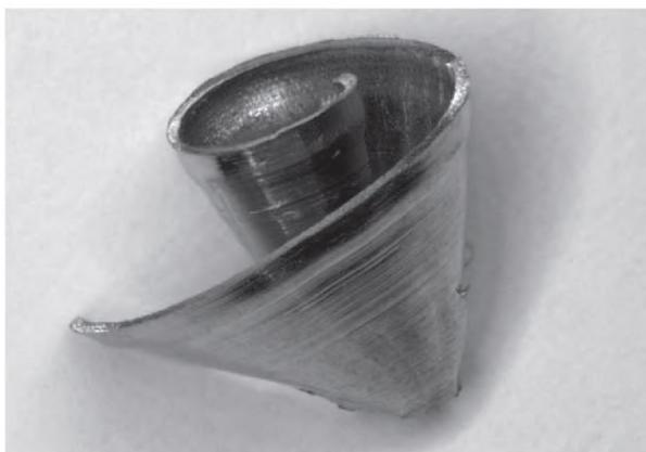
Figure 9. Chip for central insert
