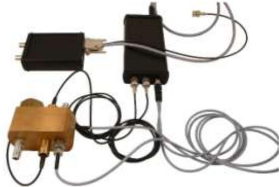
Fig. 4. Measurement setup: control unit opTim with measuring chamber and OPBOX
