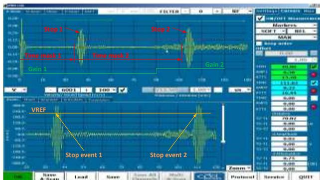
Fig. 5. Signal visualization in OPBOX for binary gas mixture with clarifications to the setup procedure of the instrument. Composition of gas mixture: methane 95.0%, nitrogen 5%
