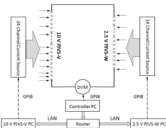
Fig. 4. Setup of an automated comparison between PJVS-W1 and the PJVS-V
