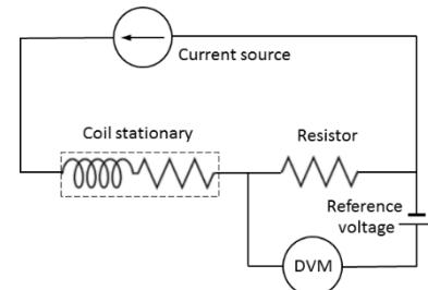
Fig. 3. Voltage measurement in force mode
