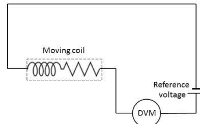
Fig. 2. Voltage measurement in velocity mode
