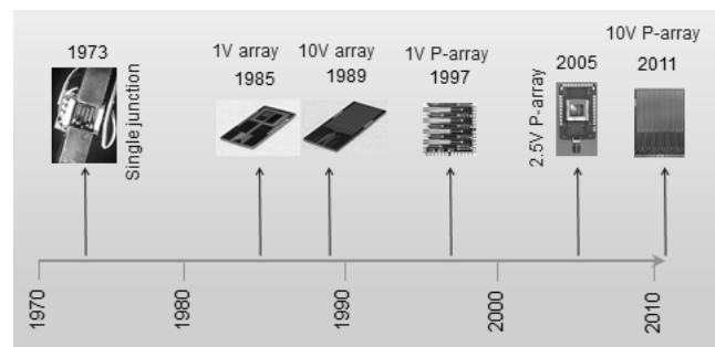
Fig. 1. Milestones of Josephson junction array development at NIST. The “array” refers to zero current bias arrays and the “P-array” refers to programmable arrays using current biased voltage steps
