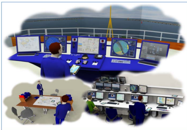
Figure 13. SAMMON System set up based on Tablet PCs within Ship Handling Simulator environment: as Bridge Version (top), Lecturer System (left) and Instructor Version (right)
