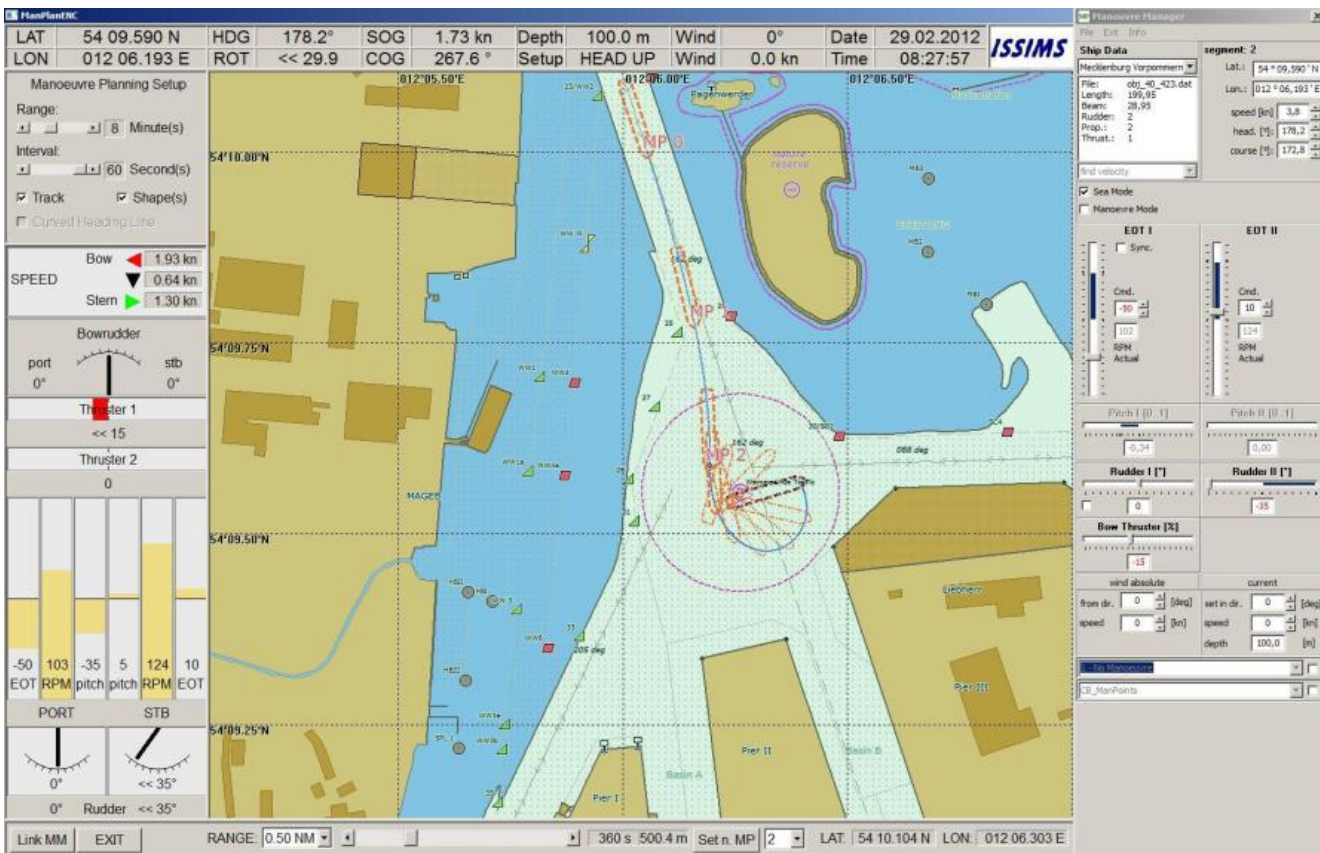
Figure 6. Planning of the next segment from MP 2 to MP 3 – complex turning and stopping with engines, rudders and thruster
