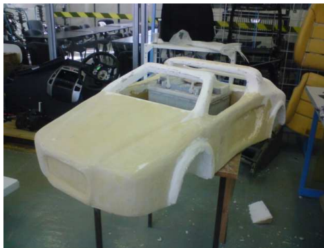
Fig. 7. Mockup fabrication (scale 1:4)
