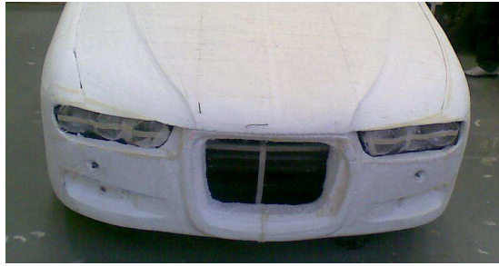
Fig. 21. Finished polystyrene model of the bumper
