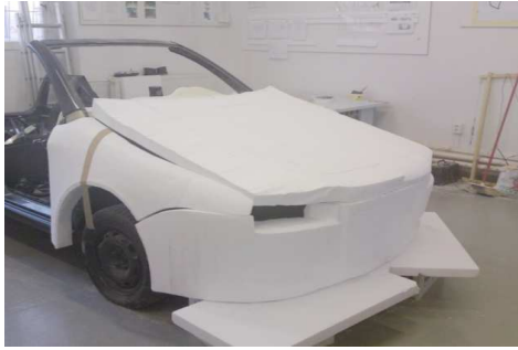
Fig. 9. Model fabrication and preparation of laminating molds (scale 1:1)
