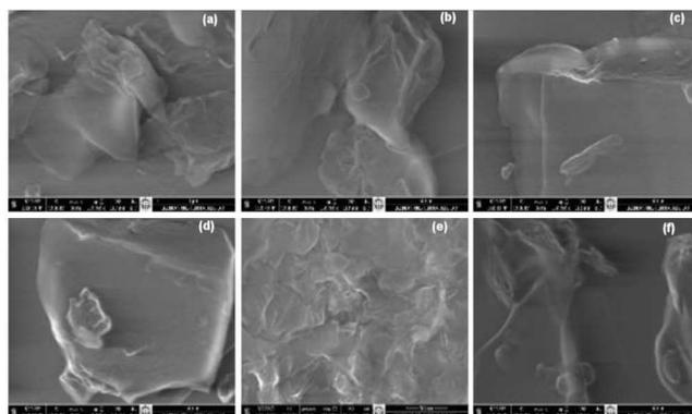
Fig. 4. The SEM images of the composites prepared using various organoclay ratios: 1 wt.% (a), 2 wt.% (b), 3 wt.% (c), 4 wt.% (d), 7 wt.% (e), and 8 wt.% (f).
