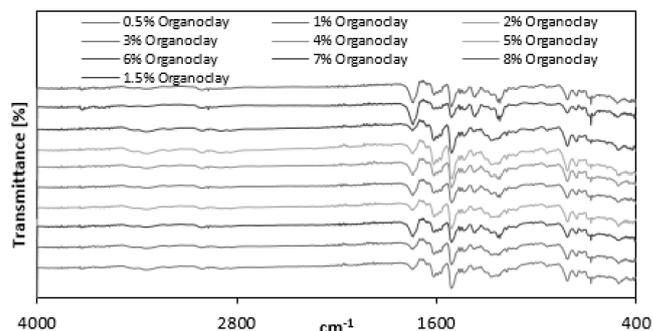
Fig. 2. FTIR spectra for organoclay-reinforced AF composites.
