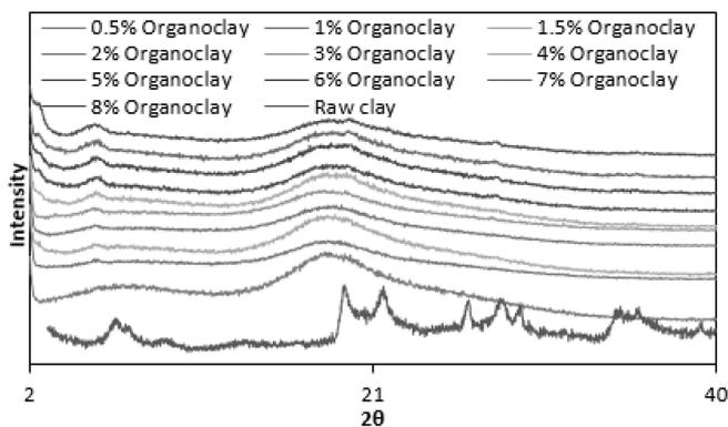
Fig. 3. The XRD patterns of organoclay reinforced AF composites and Na-Montmorillonite.
