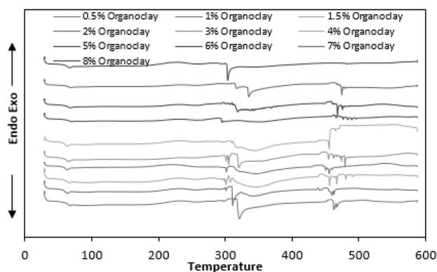
Fig. 5. The DSC thermograms of organoclay-reinforced AF composites.
