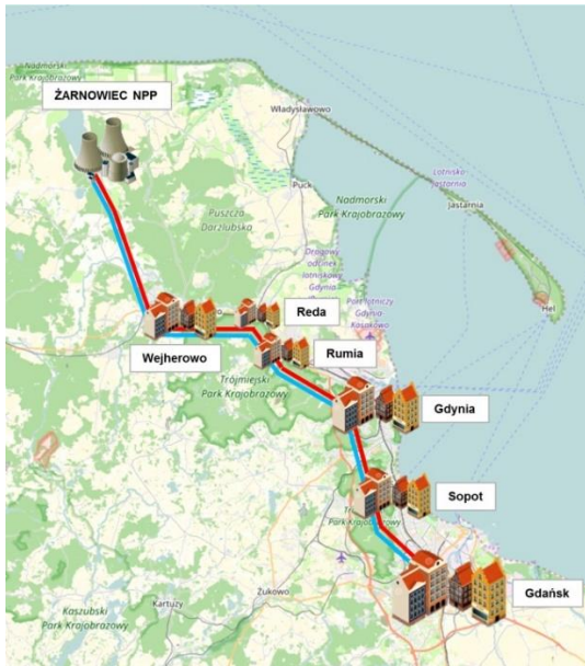
Fig. 4. The main pipeline segments in the case of Żarnowiec NPP (own elaboration; map: © OpenStreetMap contributors, CC-BY-SA 2.0 licence on www.openstreetmap.org/copyright)
