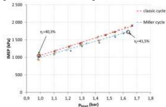
Fig. 9. IMEP as function of  $p_{boost}$  (fuel CNG)
