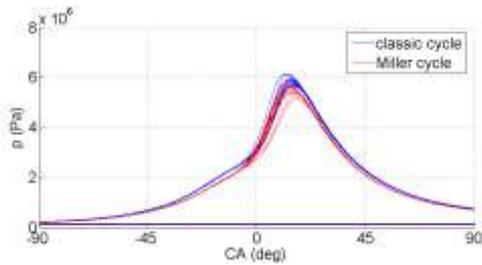
Fig. 4. Combustion pressure comparison for classic cycle engine and Miller cycle engine fuelled with coke gas (NA engine)
