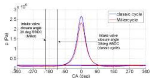
Fig. 2. Comparison of motored pressure trace for the engine with classic cycle and Miller cycle
