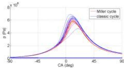
Fig 3. Combustion pressure comparison for classic cycle engine and Miller cycle engine fuelled with CNG (NA engine)
