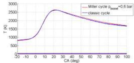
Fig. 7. Comparison of maximum in-cylinder temperature for NA classic engine and SC Miller cycle engine ( $p_{boost}=0,6$  bar), fuelled with coke gas
