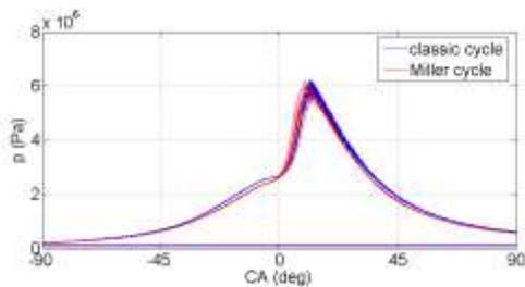
Fig. 5. Combustion pressure comparison for classic cycle engine and Miller cycle engine fuelled with hydrogen (NA engine)
