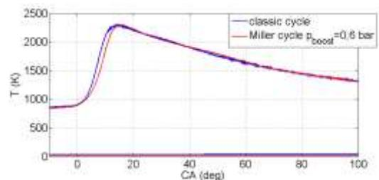
Fig. 8. Comparison of maximum in-cylinder temperature for NA classic engine and SC Miller cycle engine ( $p_{boost}=0,6$  bar), fuelled with hydrogen
