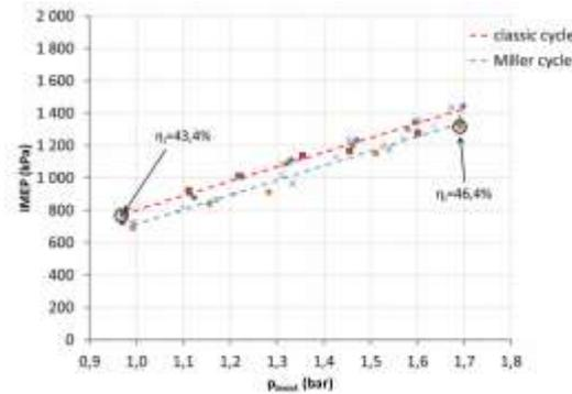
Fig. 11. IMEP as function of  $p_{boost}$  (fuel hydrogen)
