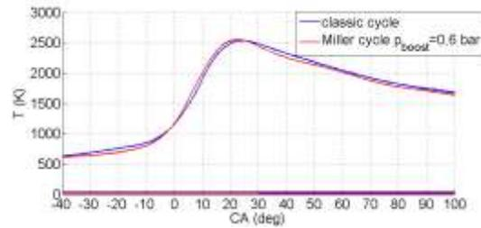
Fig. 6. Comparison of maximum in-cylinder temperature for the NA classic engine and the SC Miller cycle engine ( $p_{boost}=0,6$  bar), fuelled with CNG
