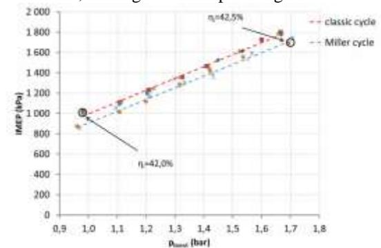
Fig. 10. IMEP as function of  $p_{boost}$  (fuel coke gas)
