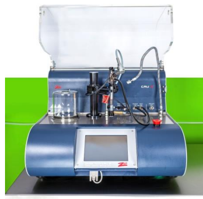
Fig. 6. Test bench for modern fuel injector testing Carbon Zapp CRU2i
