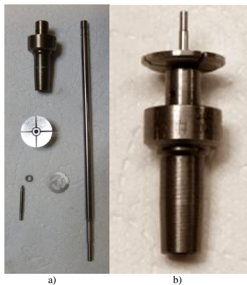
Fig. 7. a) a valve unit controlling the operation of tested CR fuel injector, b) a valve of the tested CR fuel injector with an armature plate a stator plate element
