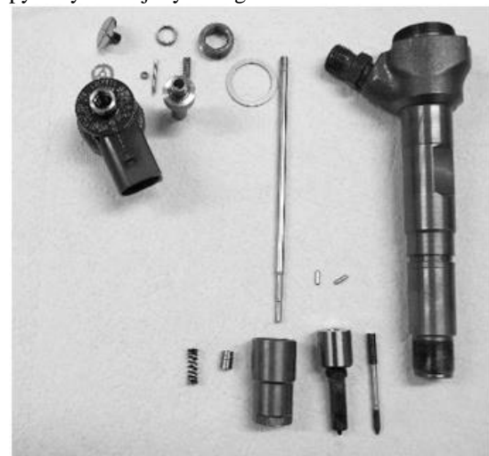
Fig. 3. Bosch fuel injector of generation 2.5, disassembled into individual components
