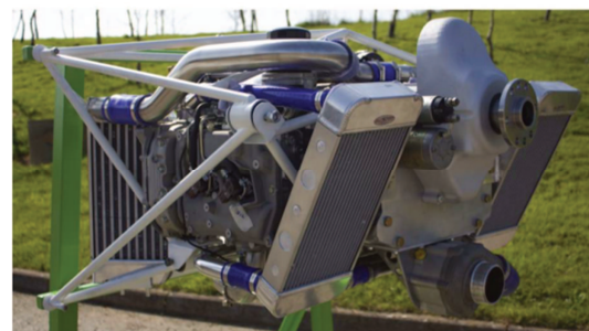
Fig. 4. CKT-240 TD diesel aircraft piston engine [8]
