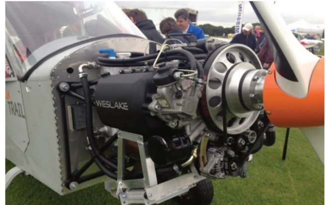
Fig. 8. Weslake A80 diesel aircraft opposite piston engine [17]
