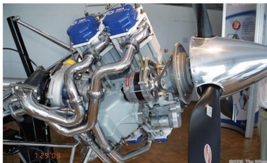
Fig. 2. Safran SR 460 diesel aircraft piston engine [16]
