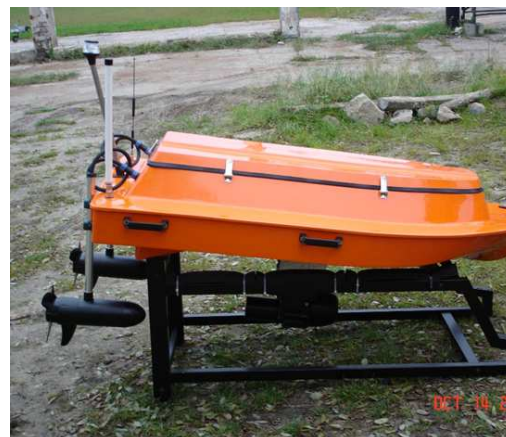
Fig. 3.9. USV Gambir hull during the first tests carried out in real conditions.
