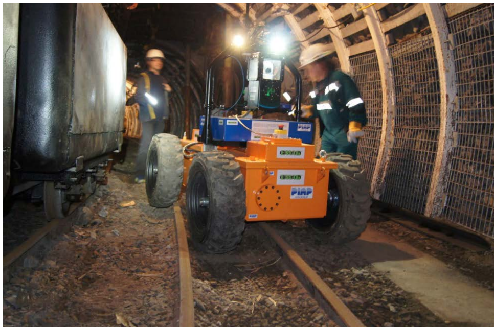
Fig. 4. MPI copes with obstacles in the mine infrastructure [14]
