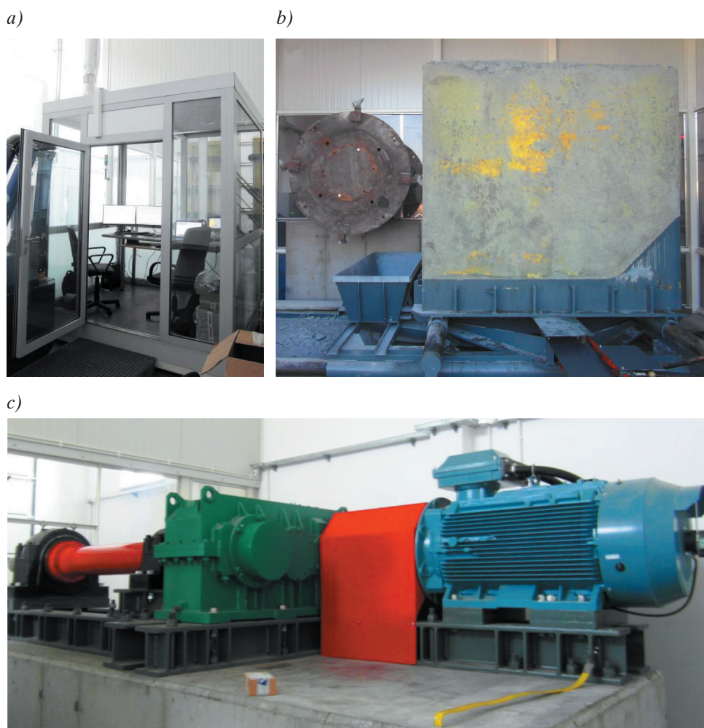
Fig. 5. Laboratory test stand to research cutting process or rotation drilling with use of single cutting tool or cutting head: a) operator ca; b) cement sample with its mounting and drive assembly and cutting head used for testing; c) drive assembly of cutting head
