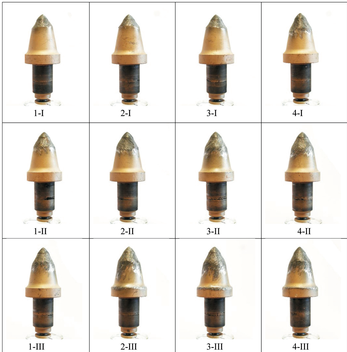
Fig. 9. Photographs of pick marked as Commercial 22 after test made-up each time rotated by 120° in relation to pick axis
