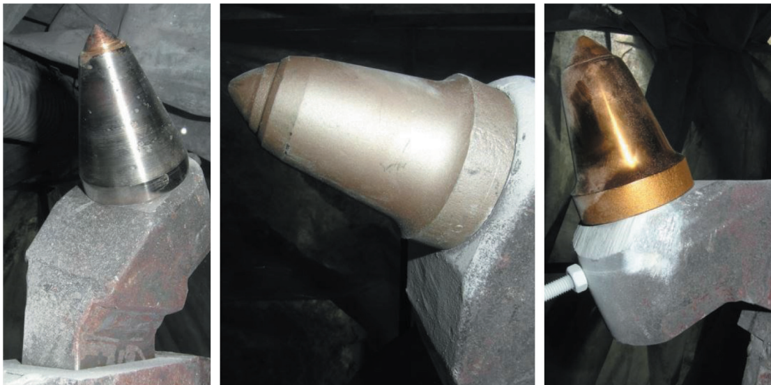
Fig. 7. Examples of tangential-rotary picks prepared for testing
