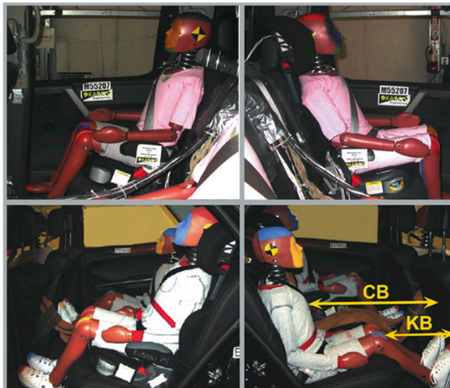
Fig. 4. The 10YO dummies in the vehicles used for tests C (top row) and F (bottom row) [28]
