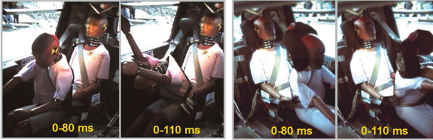
Fig. 10. Displacements of the 10YO dummies in test C at the instants of 0 ms, 80 ms, and 110 ms (based on a video record published in [28]):
