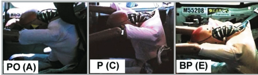
Fig. 7. Maximum tilt of dummy's head for variants PO, P, and BP (tests A, C, and E)
