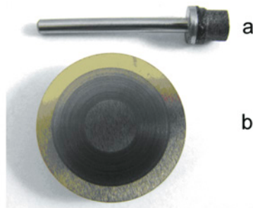
Fig. 3. Specimen (a) and counter-specimen (b), in the form of a pin and a disc, respectively
