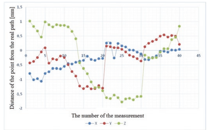
Fig. 15. Path deviation with tool rotation +20^\circ in X and Y axes in the Robcad program with the RCS Kuka_KRC1_Spot tool relative to the path measured by the Faro tracker
