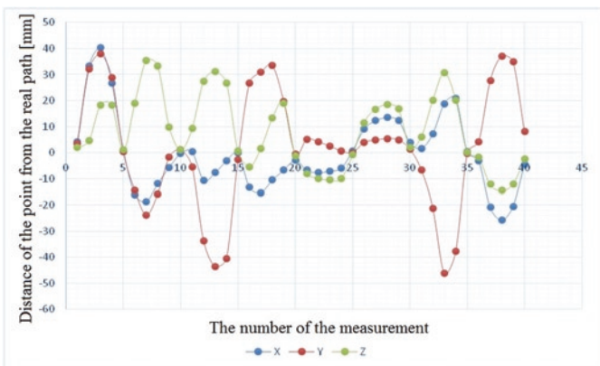
Fig. 14. Path deviation with tool rotation +20^\circ in X and Y axes in Robcad in “default” mode relative to the path measured by the Faro tracker
