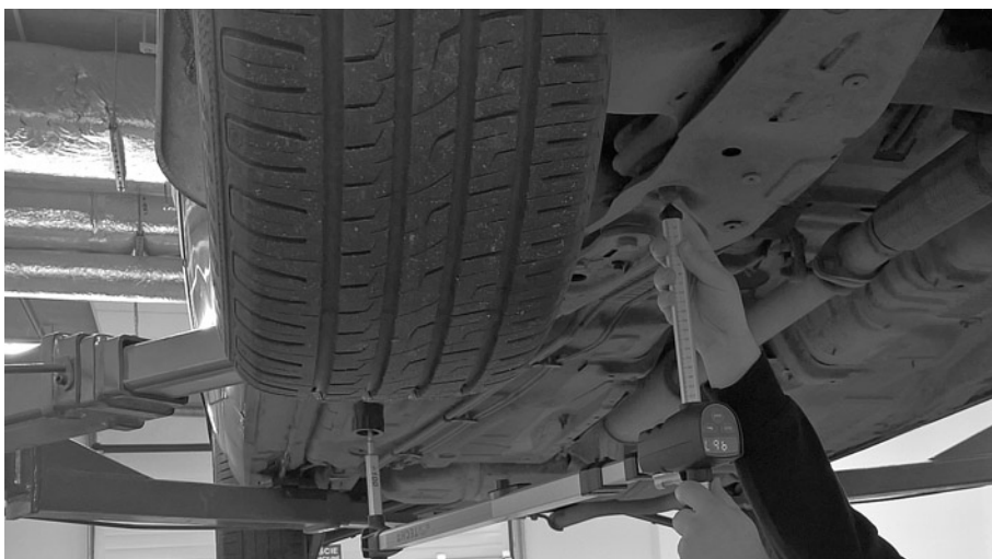
Fig. 2. Measurements of the floor panel geometry with a GYSMETER device manufactured by GYS
