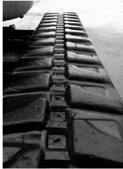
Fig. 7. The elastomeric track No. 2, the specimen in the after-operating state through the period of 1228 working hours. Numerous cracks and damages visible at the surface, the tread edges are significantly rounded and the tread is porous
