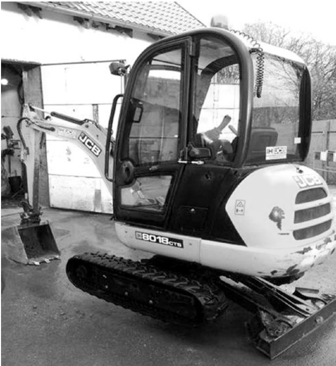
Fig. 3. Mini excavator model 8018 CTS from JCB, from which the tested elastomeric tracks came
