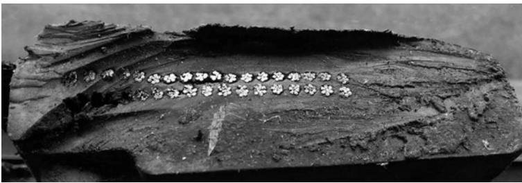
Fig. 4. Schematic diagram of the steel cord shown in Fig. 3, visible seven strands of 0,9 mm in diameter
