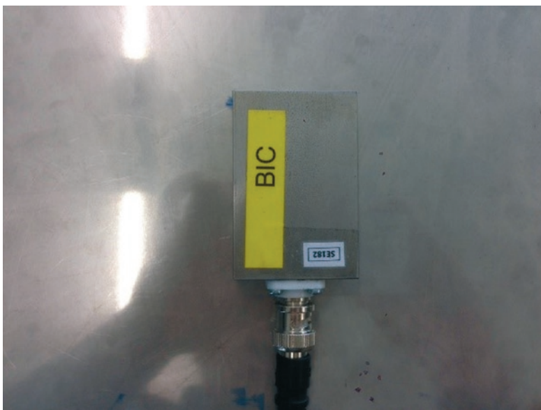
Fig. 1. Electromagnetic Acoustic Transducer manufactured by SONEMAT Limited in the UK
