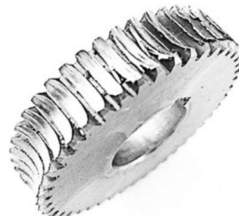
Fig. 1. Wormwheel tooth damage resulting from excessive loads.
