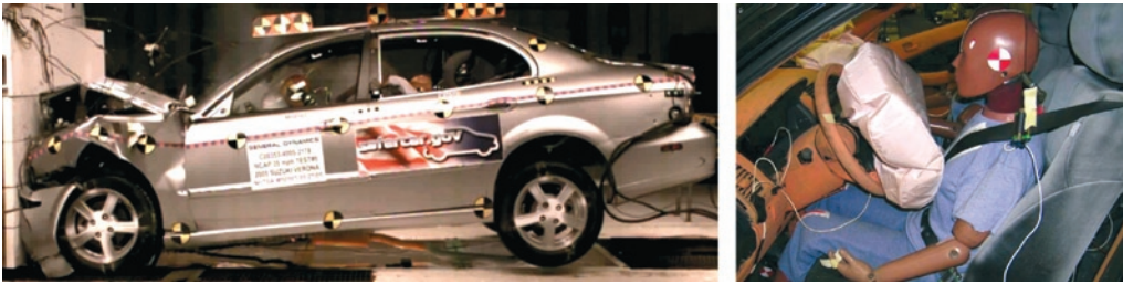
Fig. 4. Frontal impact of a car with a rigid barrier [24]
