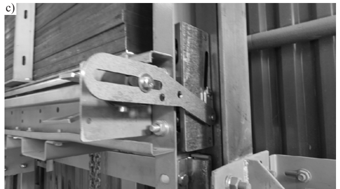
Fig. 8. The test stand: a) general view of the stand for experimental test, b) the progressive gear with the loading system in the neutral position, c) the progressive gear with the loading system at a given load
