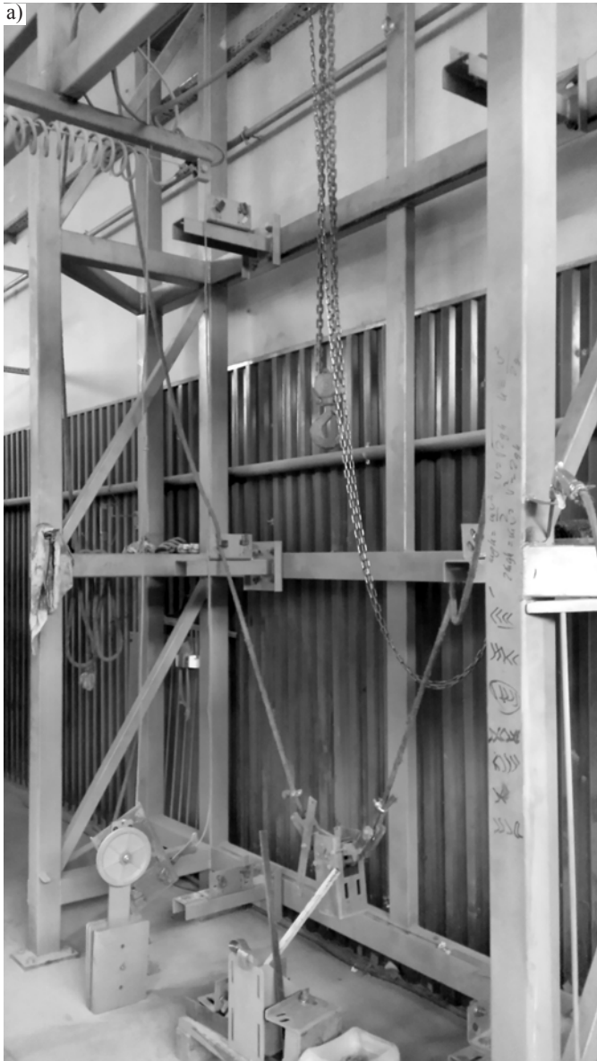
Fig. 8. The test stand: a) general view of the stand for experimental test, b) the progressive gear with the loading system in the neutral position, c) the progressive gear with the loading system at a given load
