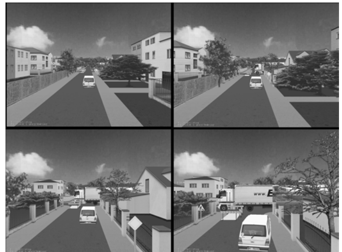
Fig. 2. Case study sample, risk of 1.8 s duration, vehicle speed 60 km/h, distance from an obstacle 30 m, the attempt ended without collision
