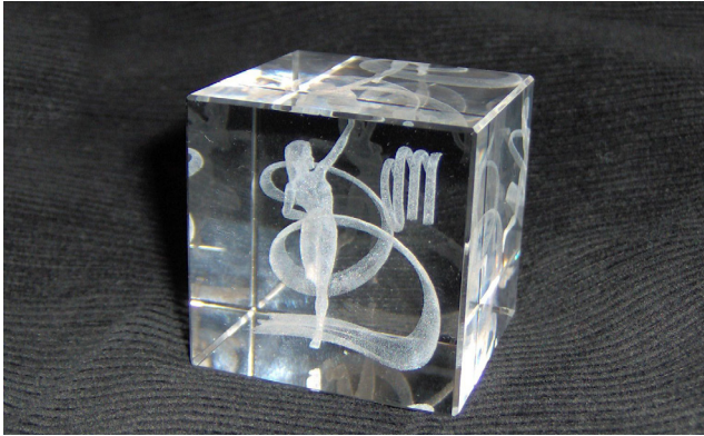
Figure 1 Example of 3D object engraving in glass (dimensions: 40 x 40 x 40 mm, 15777 points)
