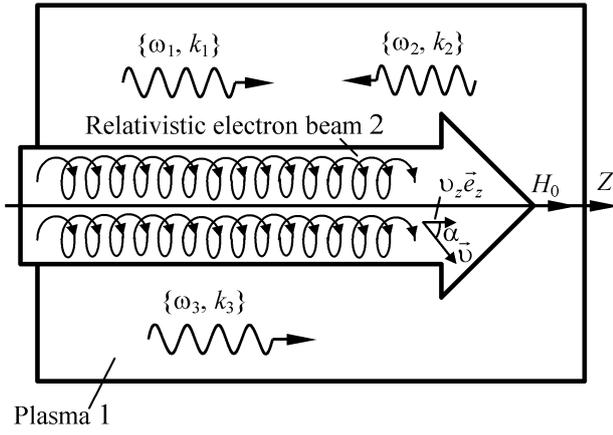
Fig. 1. Schematic diagram of the plasma-beam SFEL of dopplertron type.
