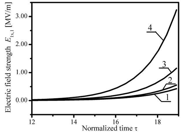
Fig. 5. Amplitudes of the first harmonic of the signal wave electric field as a function of normalized time  $\tau = t\delta\omega$  at different injection angles of the electron beam  $\alpha$  with respect to the magnetic field. Curve 1 corresponds to the injection angle  $\alpha = 0^\circ$ , curve 2 corresponds to  $\alpha = 10^\circ$ , curve 3 corresponds to  $\alpha = 20^\circ$ , curve 4 corresponds to  $\alpha = 30^\circ$ . The curves correspond to operating mode C.
