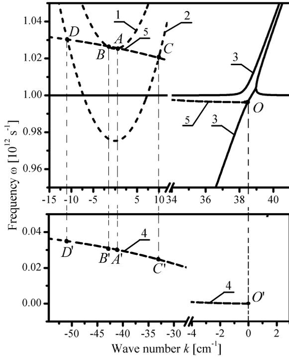
Fig. 2. Dispersion curves of the signal high-frequency electromagnetic waves (curves 1, 2) and the space charge wave (curves 3) in the plasma-beam SFEL, which were calculated for a system with the parameters given in Table.
