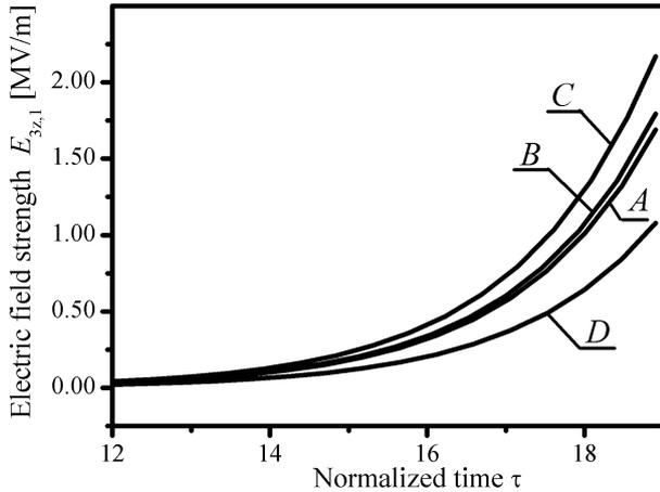
Fig. 4. Amplitudes of the first harmonic of the SCW electric field as a function of normalized time  $\tau = t\delta\omega$ . Curve A corresponds to the interaction mode A, curve B to mode B, curve C to mode C, curve D to mode D (Fig. 2).
