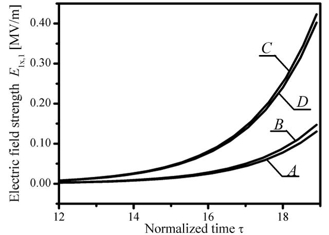
Fig. 3. Amplitudes of the first harmonic of the signal wave electric field as a function of normalized time  $\tau = t\delta\omega$ . Curve  $A$  corresponds to mode  $A$ , curve  $B$  corresponds to mode  $B$ , curve  $C$  corresponds to mode  $C$ , curve  $D$  corresponds to mode  $D$  (Fig. 2).
