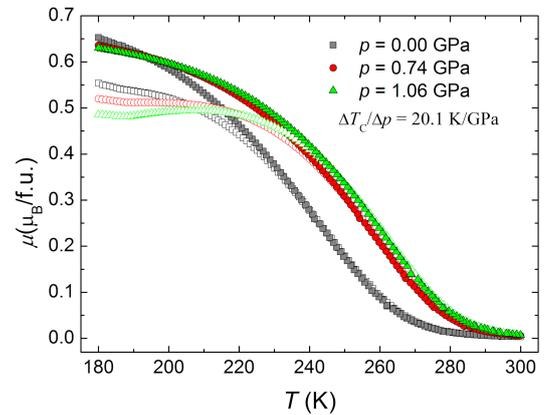
Fig. 4. ZFC and FC magnetization in vicinity of magnetic phase transition are shown at different pressures for sample with rhombohedral crystal structure.
