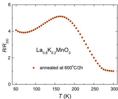
Fig. 6. Temperature dependence of the electrical resistance on the sample with rhombohedral crystal structure.
