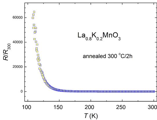
Fig. 5. Temperature dependence of the electrical resistance. The insulator type of resistivity was observed on the sample with the orthorhombic crystal structure.
