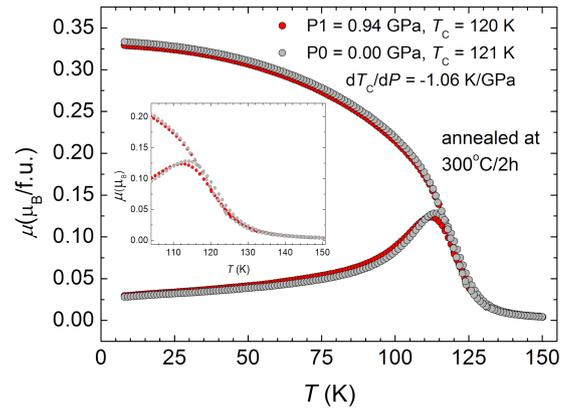
Fig. 3. ZFC and FC magnetization are shown at different pressures for sample with the orthorhombic crystal structure. The inset shows bifurcation and phase transition in detail.
