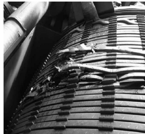
Fig. 2. Dynamic effects of short-circuit current [1].
