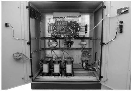
Fig. 2. The power conditioning system for SMES.
