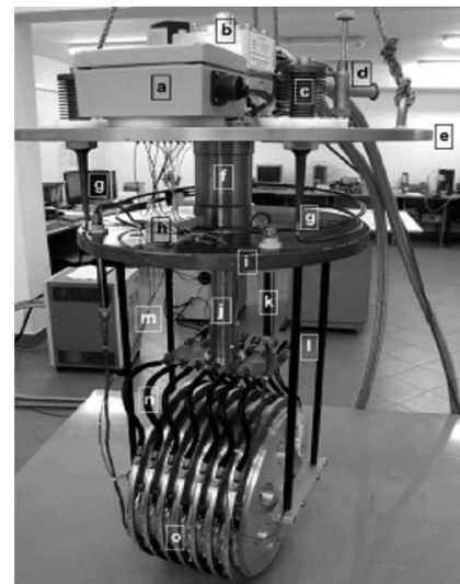
Fig. 1. Assembly of the SMES magnet: a — instrumentation socket, b — cryocooler cold head, c — current connector, d — vacuum connector, e — cryostat cover, f — 1st stage of cold head, g — copper current leads, h — thermalisation aluminium block, i — thermal shield cover, j — 2nd stage of cold head, k — HTS current leads, l — carbon-fiber tubes, m — voltage taps, n — thermal bridges, o — connections between pancake coils.
