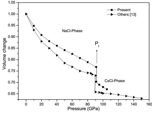
Fig. 2. Variation of volume change  $V/V_0$  with pressure.
