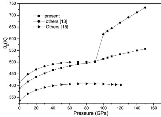
Fig. 5. Variation of Debye temperature with pressure for CdO.
