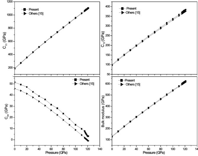
Fig. 3. Variation of SOEC's and bulk modulus with pressure.
