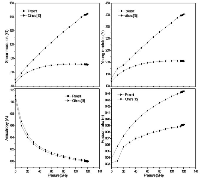
Fig. 4. Variation of shear modulus ( $G$ ), Young's modulus ( $Y$ ), anisotropy ( $A$ ) and Poisson's ratio ( $\sigma$ ) with pressure.
