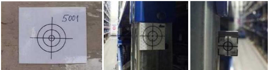
Fig. 6. Denotation of survey stations, orientations and detailed survey points
