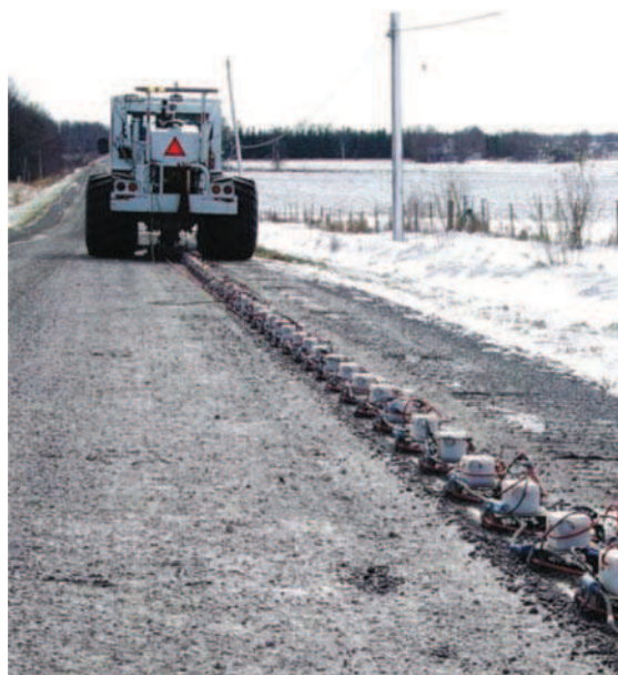
Rys. 7. Pomiary landstreamerem 3C [20] Fig. 7. Acquisition with 3C land streamer [20]
