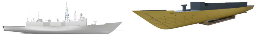
Fig. 2. Oliver Hazard Perry class frigate – actual geometry and model for tests in waves
