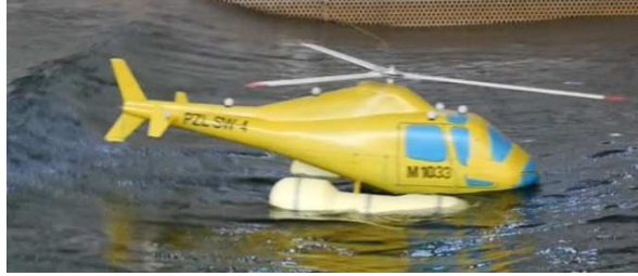
Fig. 7. Experimental evaluation of the helicopter motion in waves in model scale
