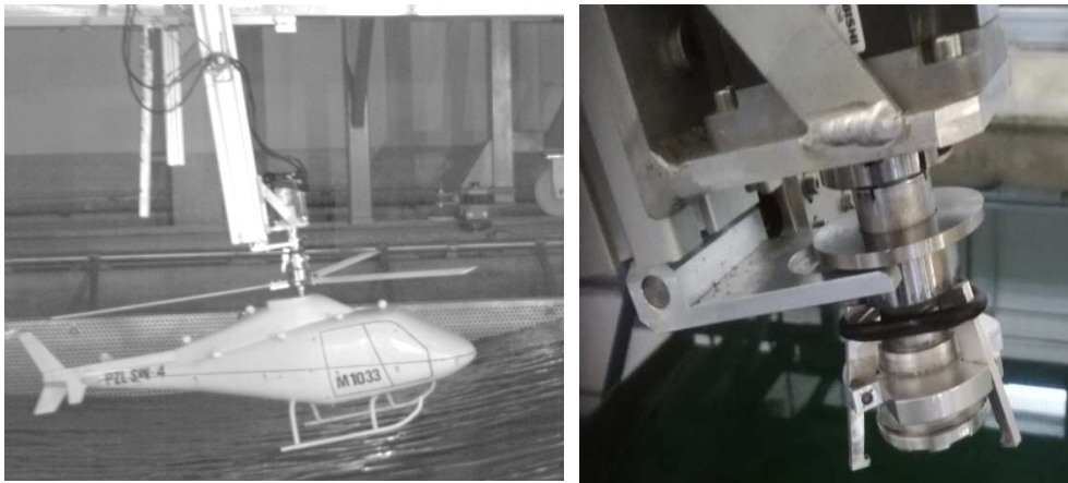
Fig. 13. Measurement stand for ditching model tests, details of releasing mechanism
