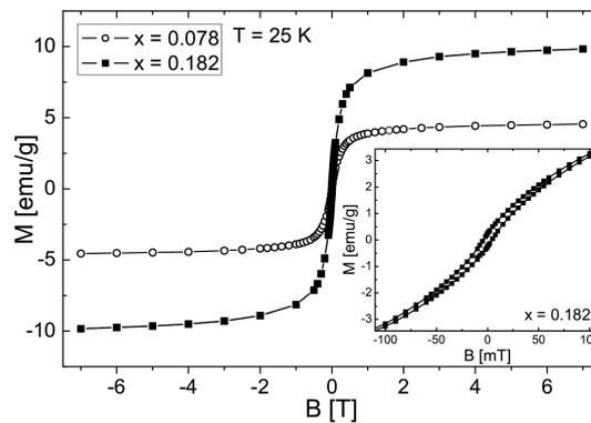
Fig. 2. The magnetization  $M$  as a function of the applied magnetic field  $B$  measured at isothermal conditions ( $T = 25$  K) for the  $Zn_{1-x}Mn_xGeAs_2$  samples (chemical composition  $x$  shown in legend).
