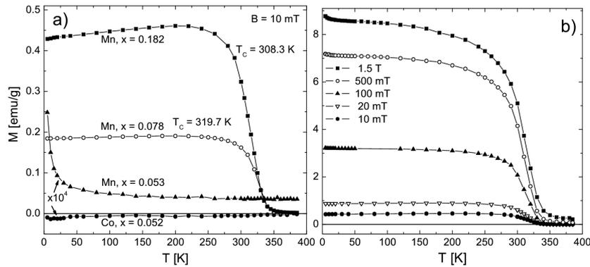
Fig. 1. The magnetization  $M$  as a function of temperature: (a) measured for the  $\text{Zn}_{1-x}(\text{Mn,Co})_x\text{GeAs}_2$  samples with different chemical compositions (labels), and (b) measured using different applied magnetic fields (legend) for the  $\text{Zn}_{0.818}\text{Mn}_{0.182}\text{GeAs}_2$  sample.
