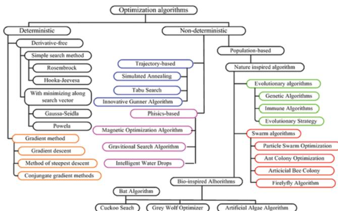
Fig. 1. The classification schema of the optimization algorithms
