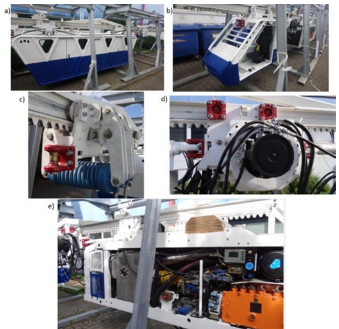
Fig. 2. Components of the suspended monorail on the testing track: a) personnel cabin, b) operator's cabin, c) breaking trolley, d) gear drive with built-in multi-disk brake, e) machinery part [7]
