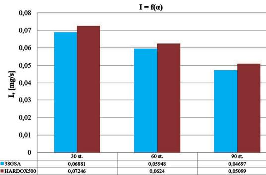
Fig. 6. Summary of 38GSA and Hardox 500 steel rate of erosion at three impact angles of particles' jet α = 30°, 60°, 90°
