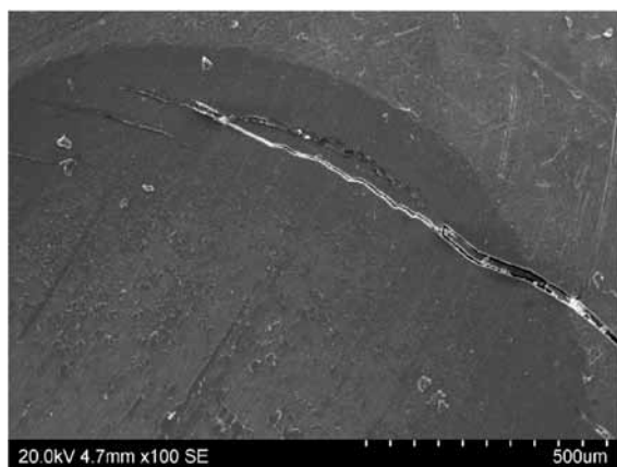
Fig. 4. SEM image of the border zone between the defect and the area before the wear test in the Enamel Plus HRi Function composite
