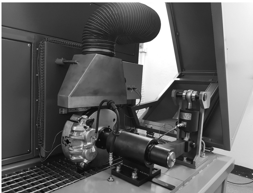
Fig. 2. Brake setup of the Iveco Daily III Van
