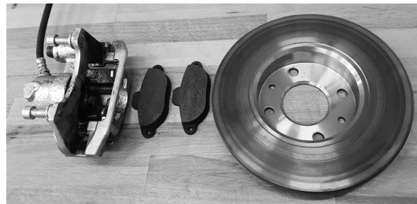
Fig. 5. The tested brake components of Cinquecento vehicle Rys. 5. Zestaw hamulca od samochodu Cinquecento
