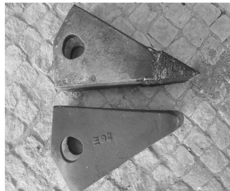
Fig. 6. Ripper with padding weld (top) and without padding weld (bottom)
