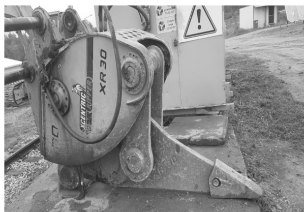
Fig. 12. Vibration ripper before installing on the KOMATSU 800LC excavator
